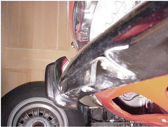
USA Cars – Bracket mounted to bumper
