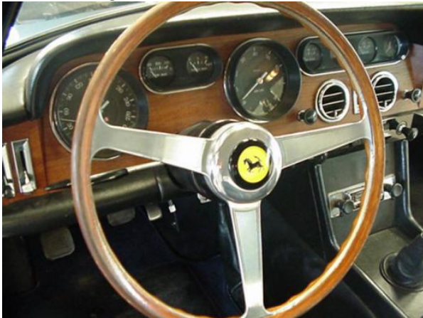
F (fog) switch with washer in place of ignition in dash
