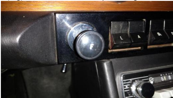
F (fog) switch with washer in place of ignition in dash
