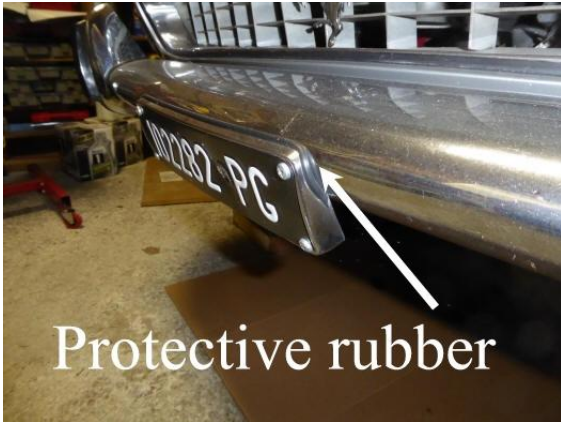
USA Cars – Bracket mounted to bumper
