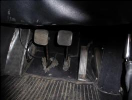
Series I through floor pedals (Note, torn boot)
